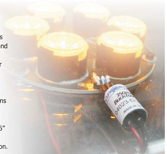
04023 BuckToot LED Driver Module powering (6) Luxeon I LEDs in series ( V_{IN} \geq 24V )
