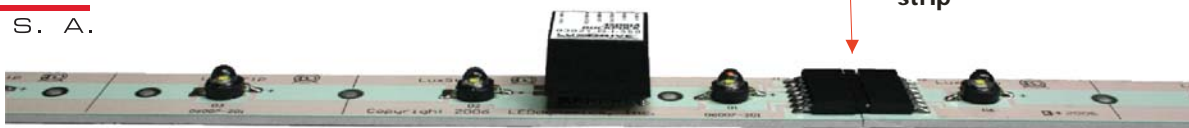
Figure 2 3021 BuckPuck powering (6) LUXEON LEDs in series ( V_{IN} = 24VDC ) and end-feeding another strip
